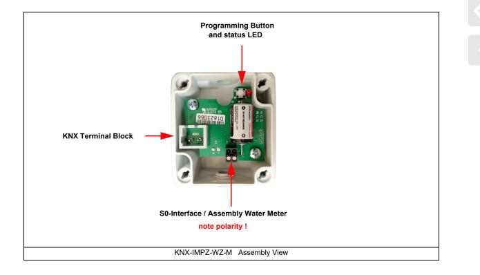
The Counter-Modul **KNX-IMPZ-WZ-M** is for outdoor and indoor areas. It fulfills protection class IP54/65. Mounting is done on wall through 2 screw holes.
