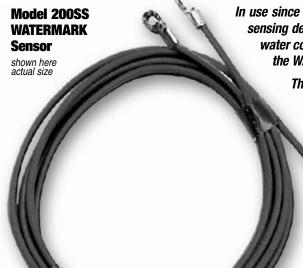
In use since 1978, the patented WATERMARK sensor is a solid-state electrical resistance sensing device that is used to measure soil water tension. As the tension changes with water content the resistance changes as well. That resistance can be measured using the WATERMARK Sensor.
